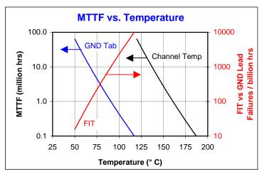
As can be seen from the MTTF values above, the predicted failure rate is still above 1 million hours, even at operating temperatures up to  $+90^{\circ}$  C (corresponding to channel temperatures of  $+160^{\circ}$  C). Also note that these MTTF estimates are a lower bound as the accelerated testing never resulted in 50% failures.
